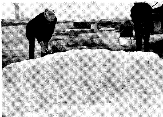
Figure 1. Foam on ammonia spill tests in progress.
